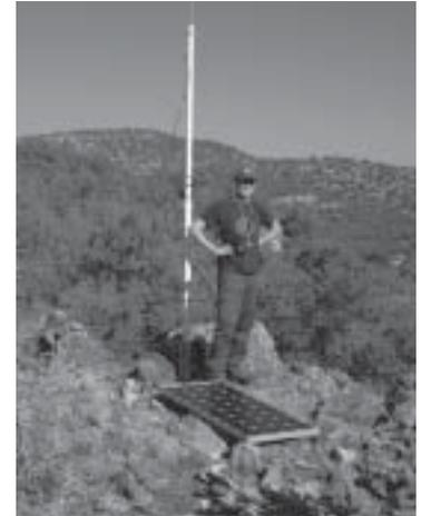
*TA Chris Hager standing by the wireless network setup. Students communicated computer-to-computer through a router powered by batteries and solar panel.*
